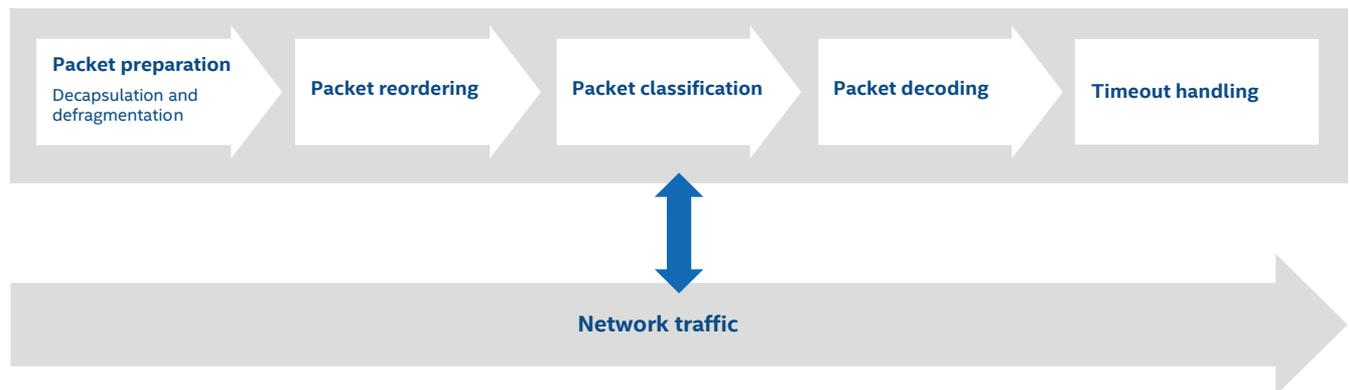
**Figure 2.** Five processing stages of R&S®PACE 2 architecture.
