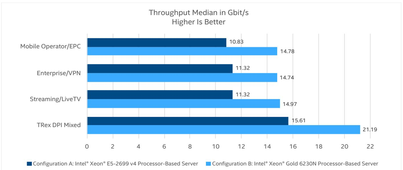
Figure 3. Configuration A and Configuration B throughput per network traffic profile. Measured on 1 logical core.
