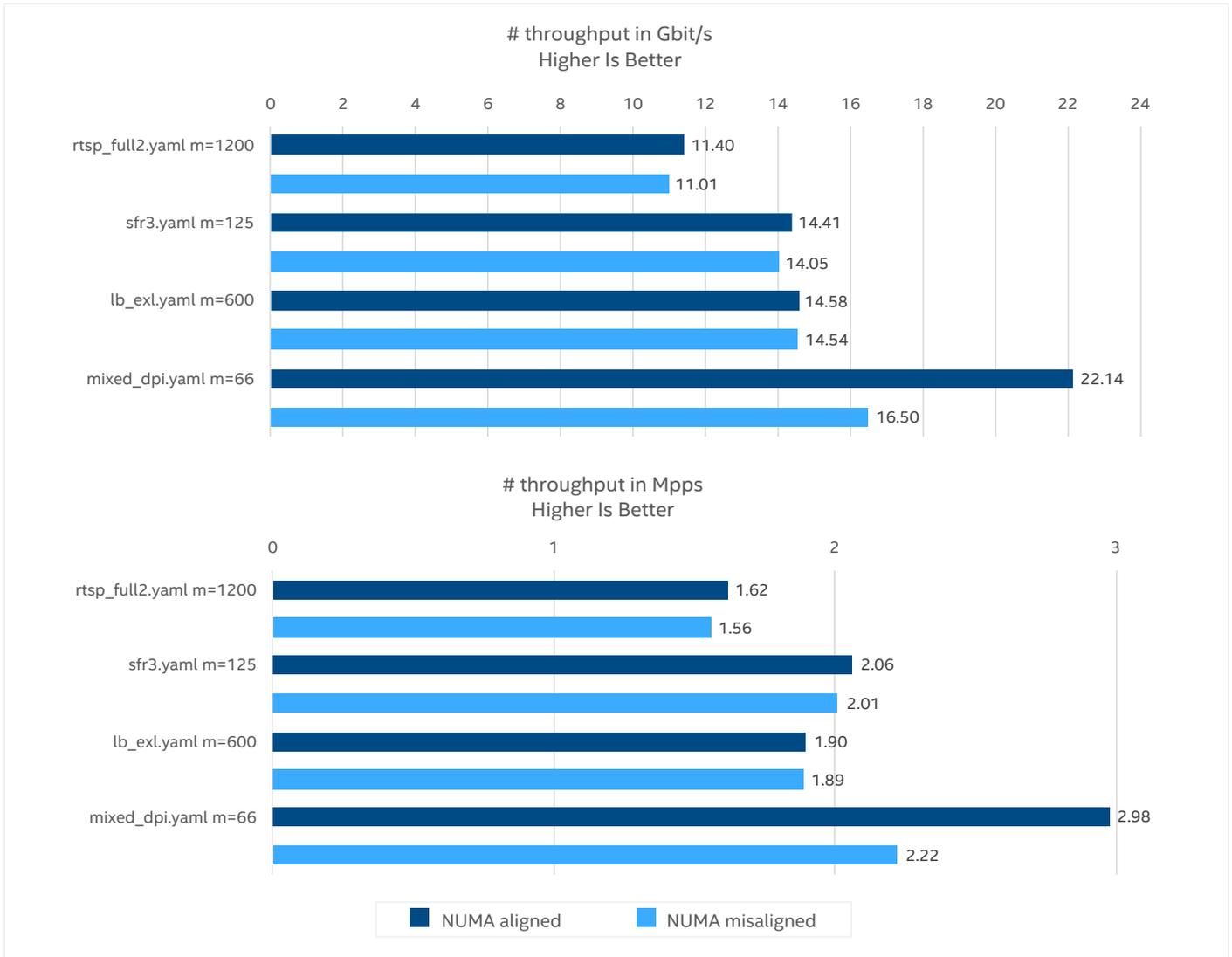
Figure 5. Test 2 results measured in Gbps and Mpps. Measured on 1 logical core.
