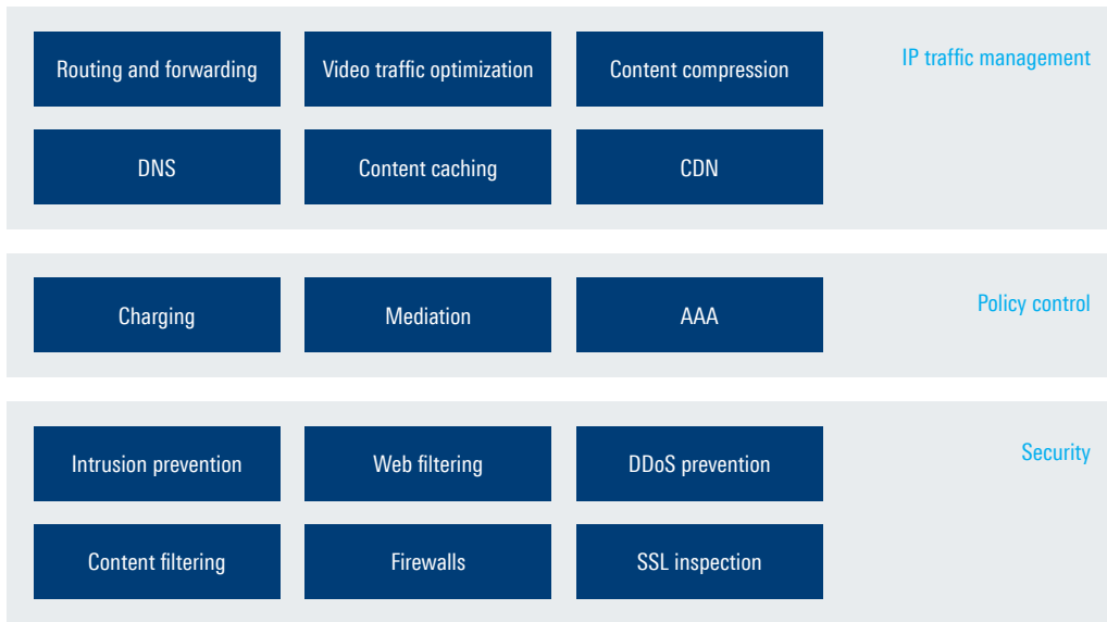
Traffic management, policy control and security functions/subsystems in mobile core networks
